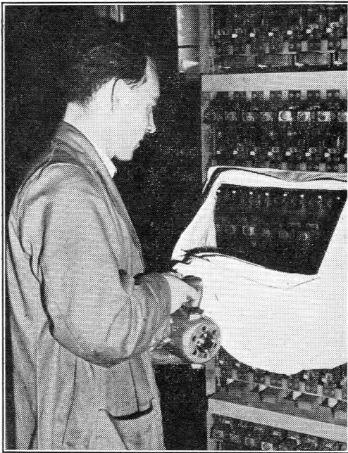
FIG. 3.—THE FRONT SHROUDING BAG WITH PLASTIC WINDOW.
