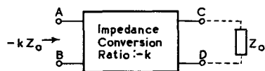
FIG. 1.—COMBINATION OF A NEGATIVE IMPEDANCE CONVERTER (BCD) AND A PASSIVE IMPEDANCE ( Z_0 ) TO GIVE NEGATIVE IMPEDANCE.
