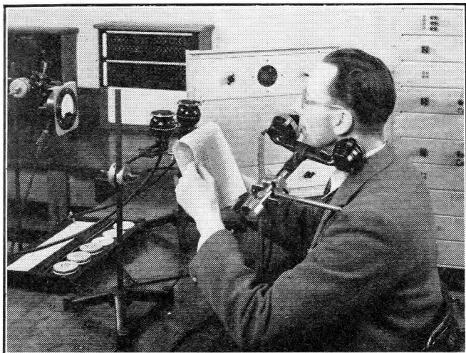
NOTE: The list of speech sounds is spoken into the microphone under test; one of the two high-quality microphones and the level meter are used for controlling the loudness of speaking.
