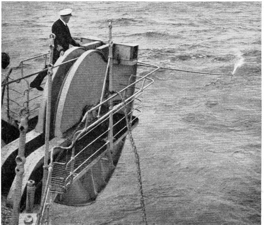
FIG. 9.—CABLE PAY-OUT OVER THE STERN SHEAVE.
