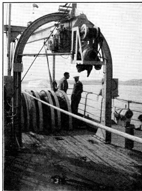
FIG. 12.—OVERHEAD GANTRY AND ELECTRIC HOIST FOR RIGID REPEATERS.
