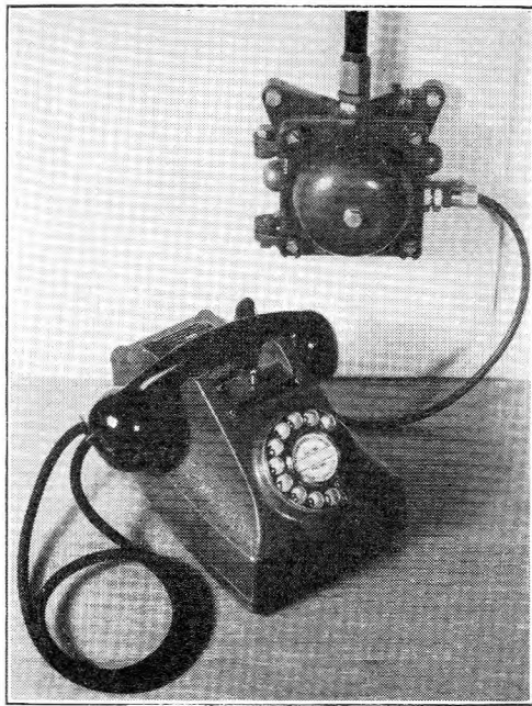
FIG. 2.—FLAMEPROOF TABLE TELEPHONE AND BELL.
