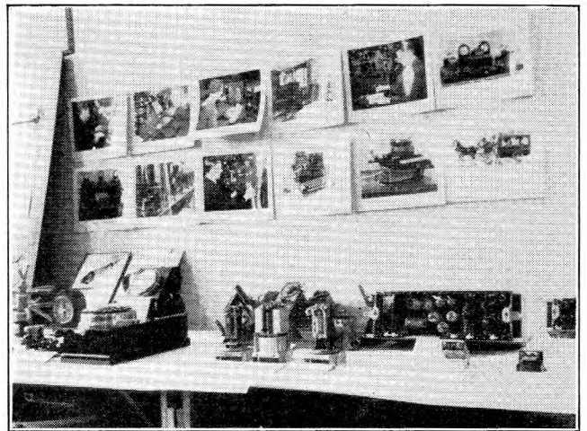
PART OF THE TELEGRAPH SECTION SHOWING "ABC" INSTRUMENT ON LEFT AND V.F. TELEGRAPH PANELS ON RIGHT.
