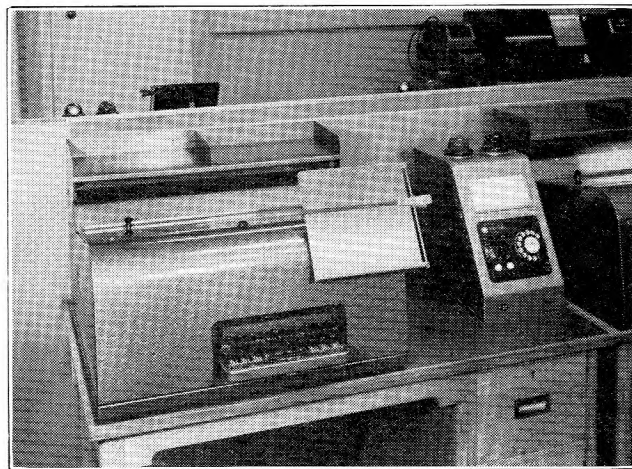
FIG. 1.—TYPICAL TELEPRINTER NO. 7D POSITION WITH SIGNALLING UNIT, TG, No. 20.
