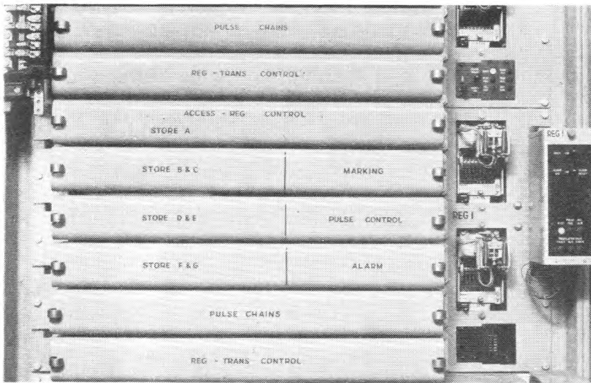
FIG. 2—INCOMING ELECTROMECHANICAL REGISTER FOR DIRECTOR AREAS
