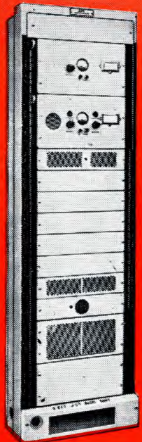
5 circuit V.H.F. junction radio terminal equipment.
