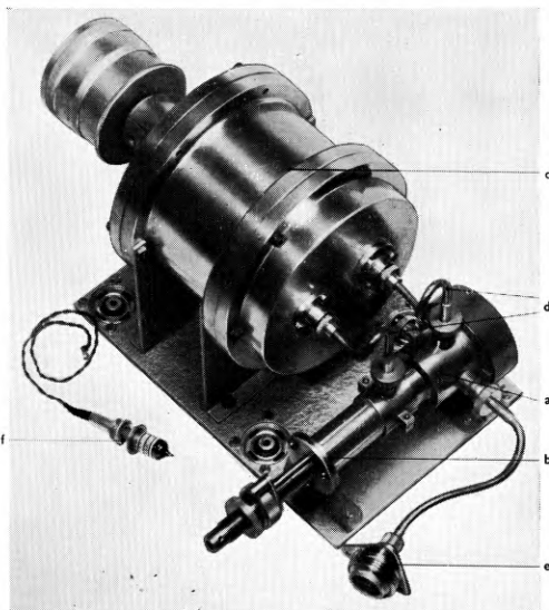
(a) Anode line of amplifier (c) Control cavity (e) Oscillator output (b) Cathode line of amplifier (d) Coaxial coupling leads (f) Microwave triode valve
