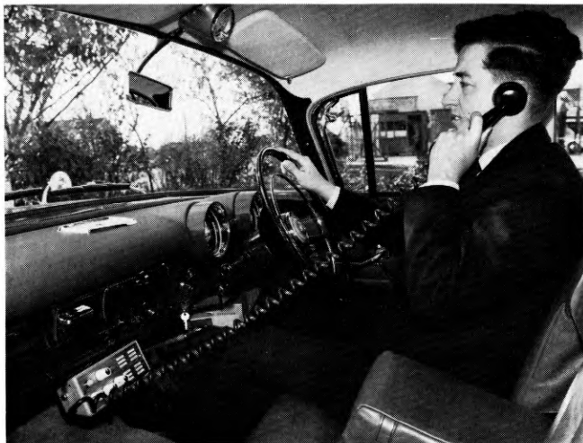
FIG. 8—CONTROL POSITION IN VEHICLE
