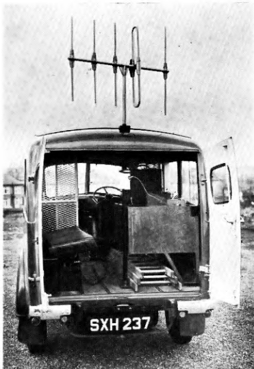
FIG. 3—INTERIOR OF VEHICLE SHOWING OPERATING POSITION, APPARATUS CABINET AND AERIAL SUPPORT
