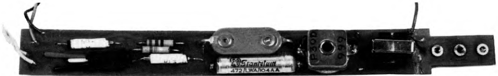
FIG. 2.—TRANSISTOR AMPLIFIER COMPONENTS MOUNTED ON INSULATING STRIP
