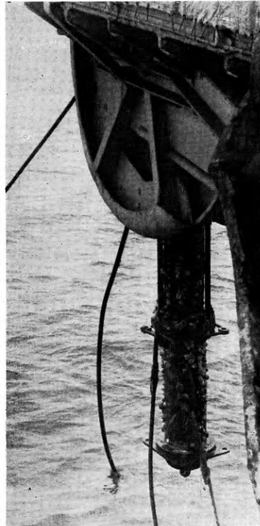
FIG. 1—RECOVERED FAULTY REPEATER UNDER BOW SHEAVES
