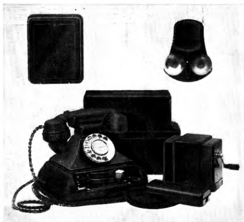
(b) Apparatus required at main station when Bell Set No. 44 is used
