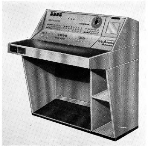
FIG. 6—G.E.C. NO. 4 CORDLESS SWITCHBOARD
