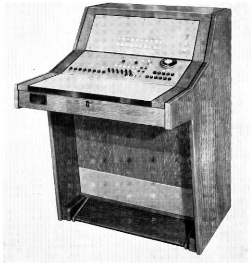
FIG. 5—A.T.E. NO. 4 CORDLESS SWITCHBOARD
