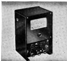
The Post Office Tester is a multi-range meter used for making tests on subscribers' apparatus and lines.
