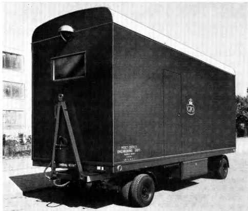
FIG. 2—MOBILE SWITCHING UNIT VEHICLE
