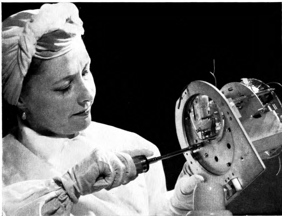
Assembly of a supervisory unit for a Submerged Repeater
