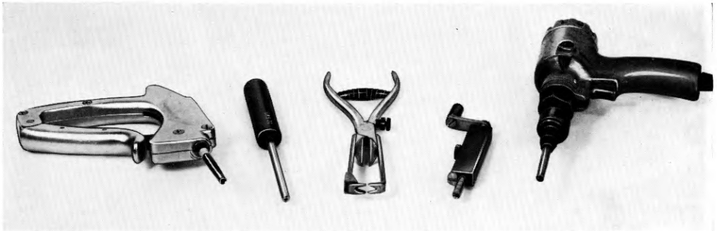
The tools are, from left to right: (i) Pistol-strip wrapping tool (ii) Direct-action wrapping tool (iii) Wire stripping and cutting tool (iv) Crank-handle wrapping tool (v) Electric-motor wrapping tool
