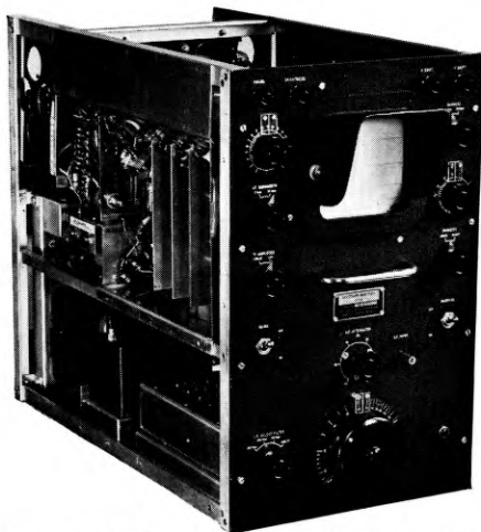
Cover removed to show 450 kc/s i.f. amplifier and deflexion amplifiers SPECTRUM ANALYSER FOR THE FREQUENCY RANGE 25–140 MC/S
