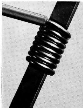
(a) Primary Wrapped Joint
