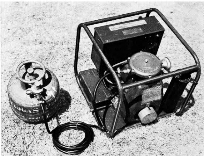
The primary pressure-regulator is mounted on the gas cylinder and the low-pressure regulator is fitted on top of the engine.
