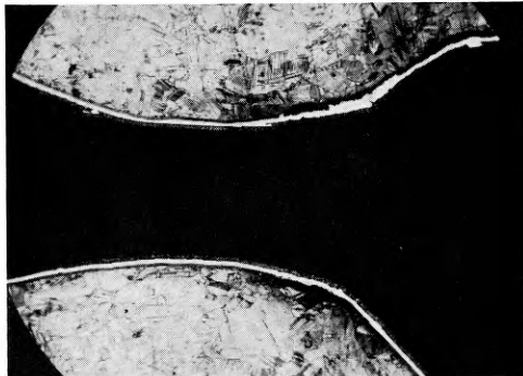
(b) Contact area showing bad adhesion. Magnification 120 times
