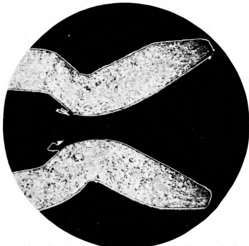
(a) Contact area etched showing bad adhesion between base metal and gold plating. Magnification 30 times
