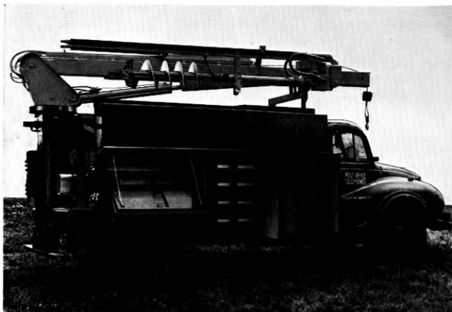
FIG. 1—THE NEW LINE-CONSTRUCTION VEHICLE
