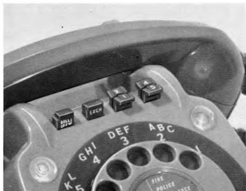
FIG. 3—PRESS-BUTTONS AND SUPERVISORY LAMPS ON INTERCOMMUNICATION TELEPHONE
