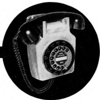
S.E.C. 711 telephone a general purpose wall instrument.
