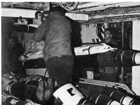
FIG. 3—LOADING THE NEXT REPEATER TO BE LAID ON TO A TROLLEY IN THE CENTRE CASTLE OF MONARCH
