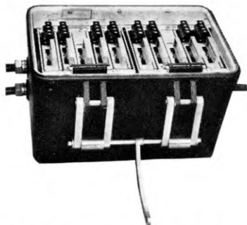
Dependent repeater housing with lid removed showing repeater units fitted for two systems.
