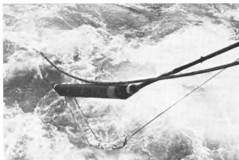
The rope used to enable repeater to by-pass the V-sheaves is slack. FIG. 4—REPEATER ENTERING THE SEA AT ABOUT 1 KNOT. PARACHUTE ABOUT TO PULL OUT OF COVER WHICH IS RECOVERED BY ROPE
