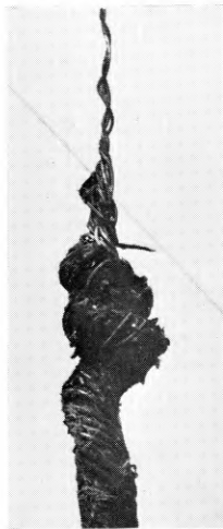
FIG. 1—FAILURE OF ARMoured CABLE CAUSED BY ROTATION DURING A REPEATER RECOVERY OPERATION
