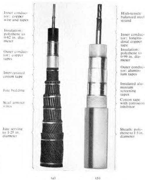
(a) Conventional (Armoured) Cable Used up to 1960 (b) Lightweight (Armourless) Cable Used 1961 Onwards
