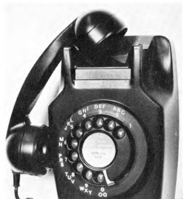
FIG. 2—"OFF-HOOK" REST POSITION FOR HANDSET
