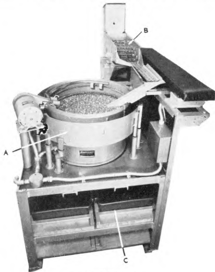
A—Second sorting unit B—Filling hopper and linear feeder C—Tray for sorted screws
