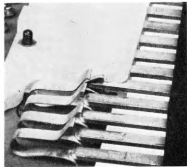
(c) Cut-way View showing Cup Springs in a Nylon Mounting Suitable for Fitting to a Printed Board
