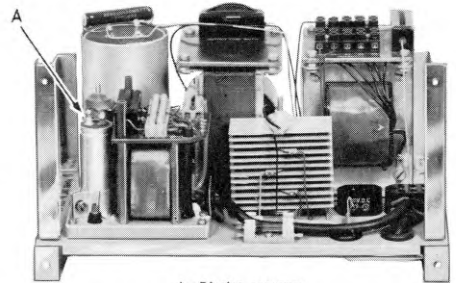
A—Ringing converter FIG. 6—CONVERTER, RINGING, No.7 MOUNTED IN POWER UNIT
