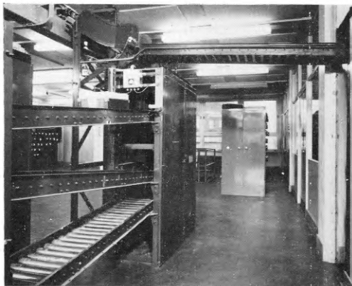
FIG. 7—GENERAL VIEW OF STORAGE RACK, SHOWING LIGHT-RAY UNIT
