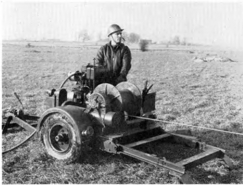
FIG. 2—MOBILE 2-TON DIESEL-ENGINE POWER WINCH
