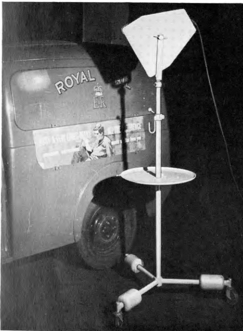
FIG. 7—THEATRICAL-TYPE PORTABLE FLOODLAMP (LAMP, ELECTRIC, NO. 21)
