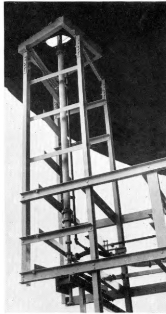
(b) Polarization Filter with Circular-to-Rectangular Waveguide Transition.
