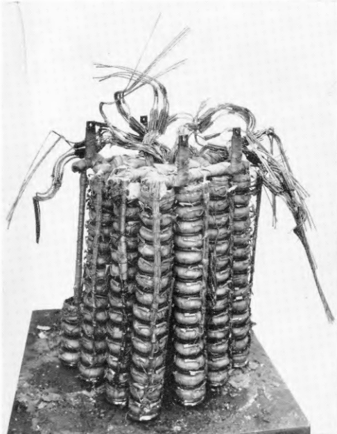
FIG. 6—COIL ASSEMBLY AFTER SURPLUS WAX HAS BEEN REMOVED
