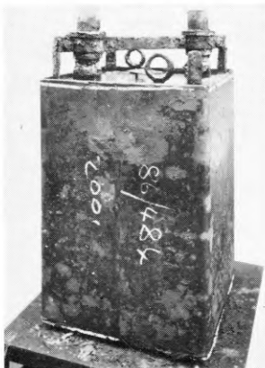
The white line round the top of the case indicates the proposed line of the cut. FIG. 3—TYPICAL WELDED CASE AS RECEIVED FOR REPAIR
