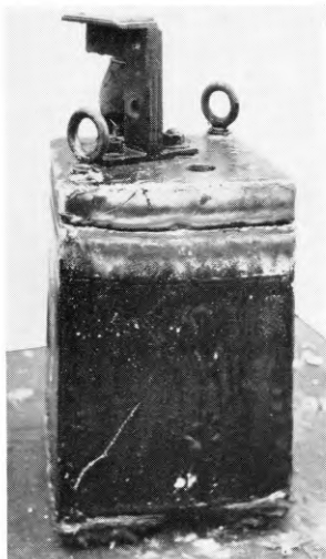
FIG. 4—MODERN SINGLE-STUB CASE OF WELDED CONSTRUCTION CUT OPEN
