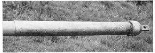
FIG. 4—DUCT, SLEEVE AND CAP READY FOR ATTACHING TO MOLEPLOUGH
