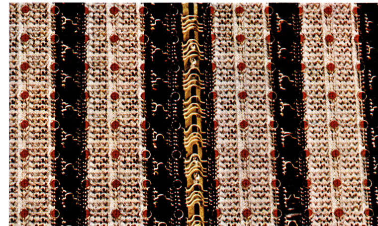
(TOP LEFT) Part of a cross-point switching frame also showing associated electronic modules. (TOP RIGHT) A sub frame withdrawn for inspection showing the method of tape wiring. (AT LEFT) Electronic modules can be arranged to revolve horizontally or swing down for inspection and maintenance. (BOTTOM LEFT) Terminal wafers may be easily withdrawn from the main block to reveal circuit components mounted within the wafer. (BOTTOM RIGHT) Frame assembly illustrating the wiring gutters used to accommodate the tape wiring.
