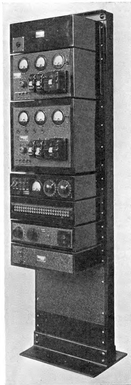
FIG. 21.—RECEIVING EQUIPMENT. GUERNSEY-MAINLAND ULTRA SHORT WAVE CIRCUIT.
