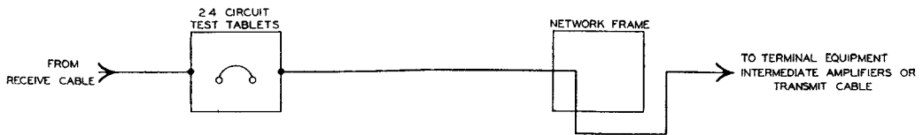
FIG. 11.—FAR-END CROSSTALK BALANCING NETWORKS. SCHEMATIC WIRING DIAGRAM.
