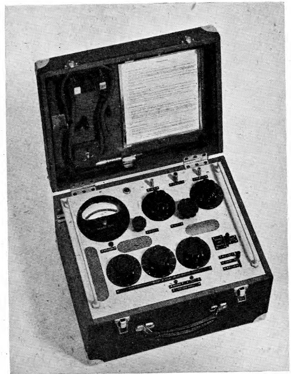
FIG. 4.—PORTABLE H.F. TRANSMISSION MEASURING SET.
