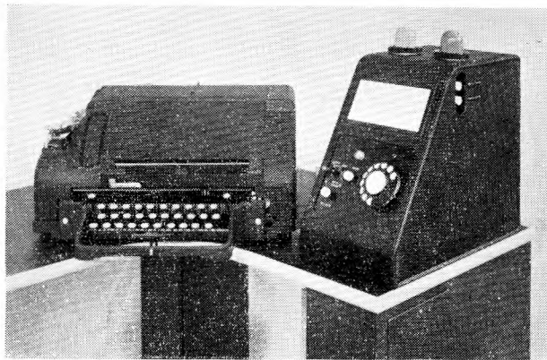
FIG. 11.—TELEPRINTER NO. 11B AND DIALLING UNIT.
