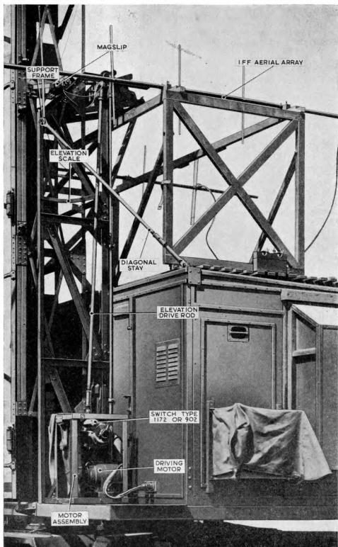
Fig. 33. R.V.461C : elevation drive mechanism
