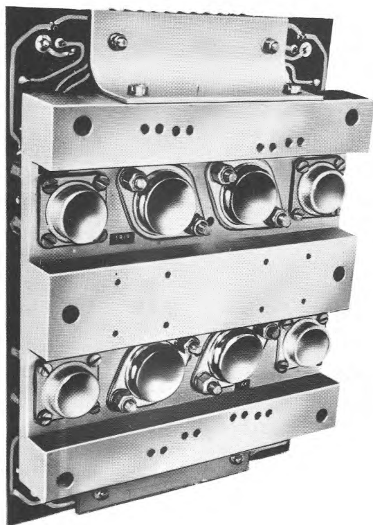
Fig.1 Deflection coil drive amplifier: general view
