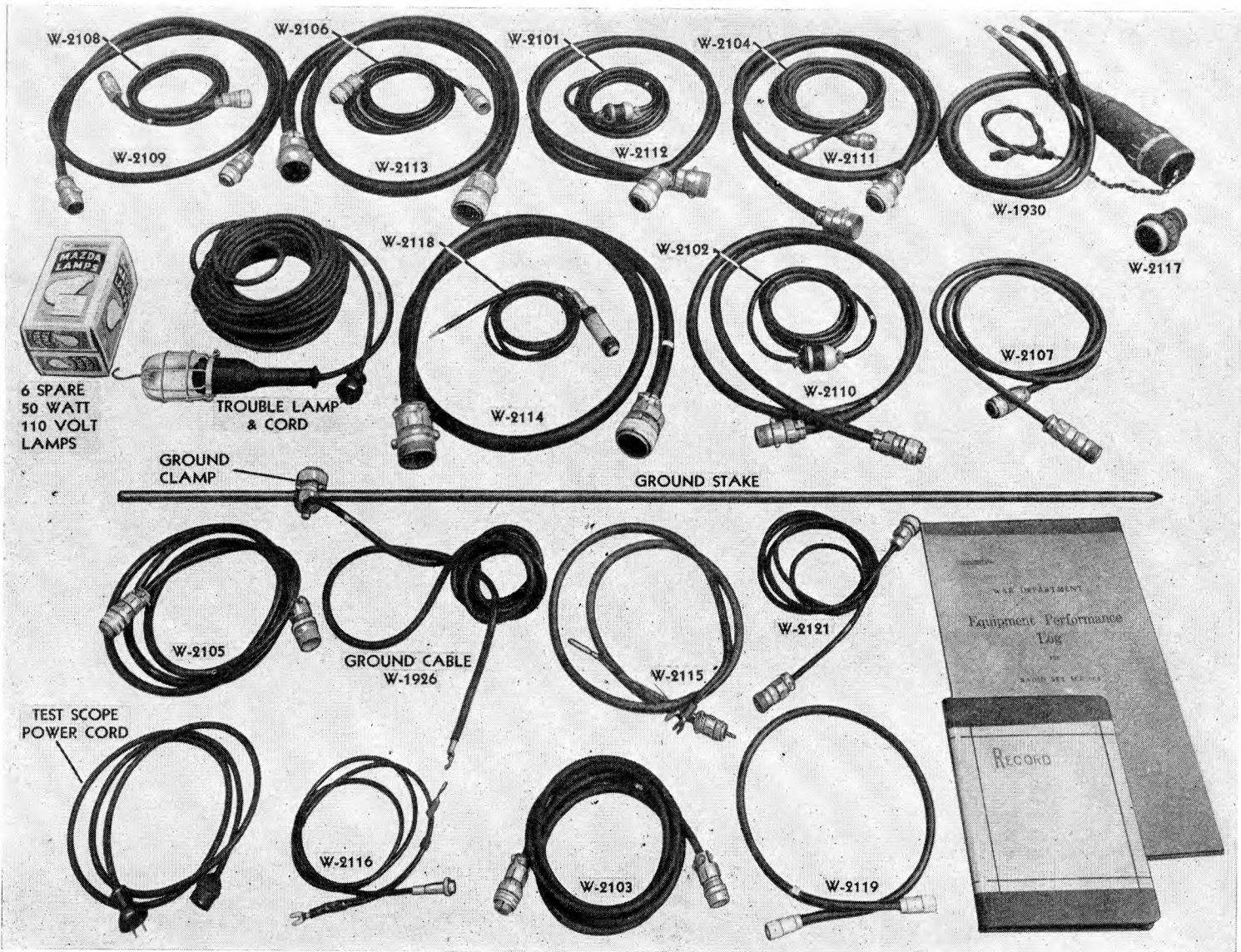
Fig. 29—Test cables provided with equipment
