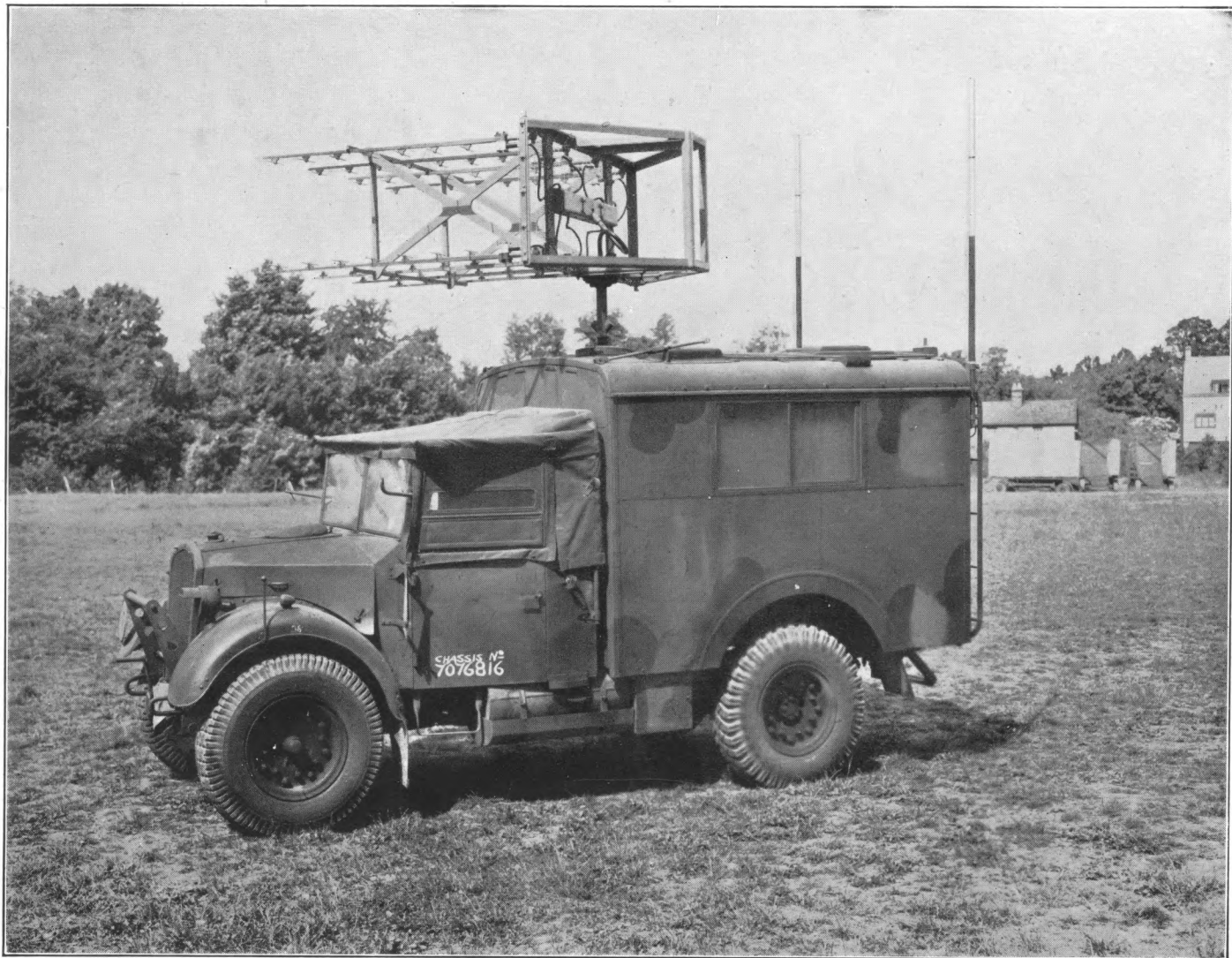
AMES Type 6 Mk. V, showing IFF Mk. III Aerials at rear of Truck
