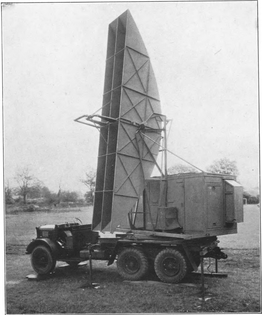
AMES Type 13 Mk. II. Aerial Vehicle (RV 461) only, showing vertical "cheese" aerial system
