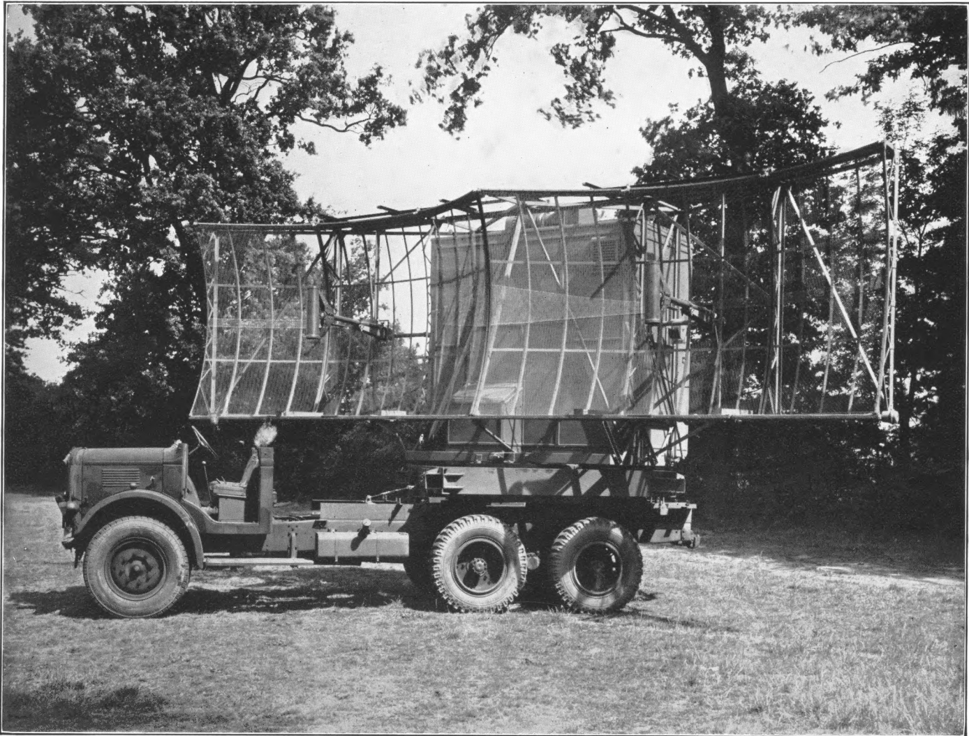
AMES Type II Mk. II (M). Prime-mover Aerial/Transmitter Vehicle (RV 433) only
