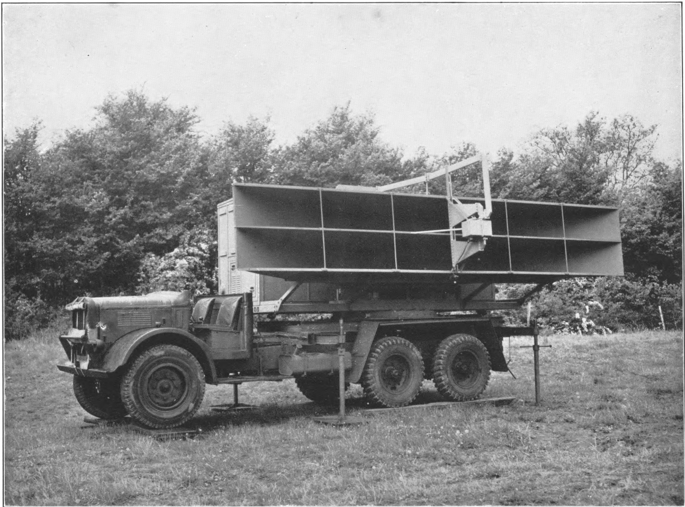
AMES Type 14 Mk. III. Aerial Vehicle (RV 462) only, showing horizontal "cheese" aerial system
