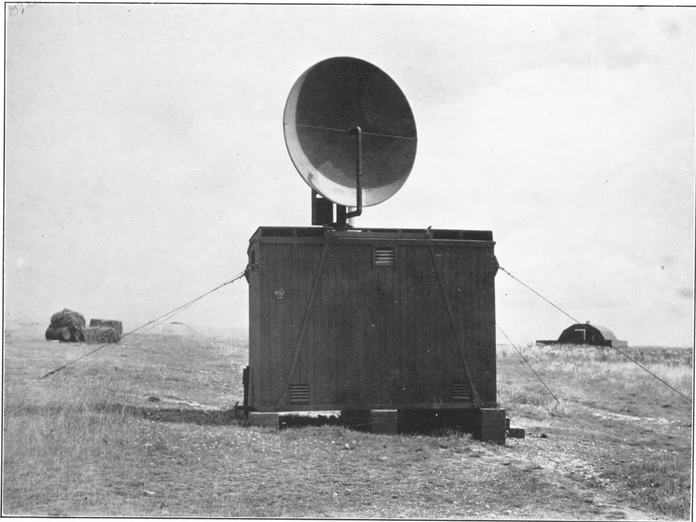
AMES Type 31 (CD No. 1 Mk. V). The AMES Type 41 (CD No. 1 Mk. V*) is essentially similar in appearance
