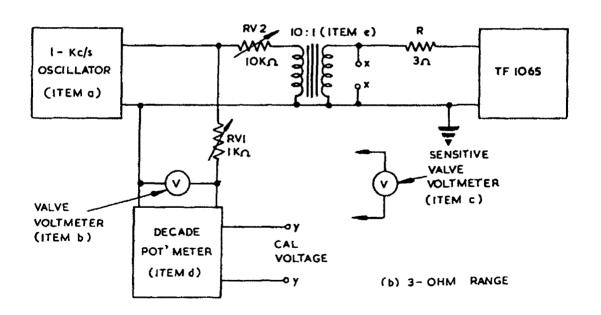
TEST CIRCUIT FOR A.F. POWER METER (SEE SECTION 4.8.2.)
