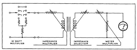
Design Limitations. The instrument is designed particularly for measurements at frequencies in the middle part of the audible band, where the impedance accuracy is high and the accuracy of power indication is limited only by that of the rectifier type meter.
