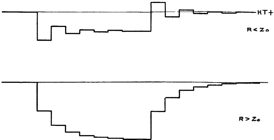
Fig. 135.—Output waveform of circuit of fig. 131 when R \neq Z_0
