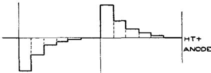
Fig. 131.—Waveforms of circuit of fig. 129, when R < Z_0
