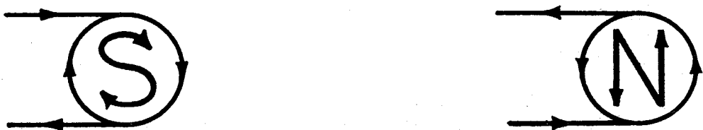
FIG. 10, CHAP. II.—Mnemonic for polarity of solenoid.
