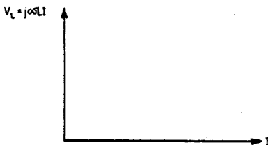
Fig. 6. PHASE ANGLE IN AN INDUCTANCE SHOWN BY 'j'
