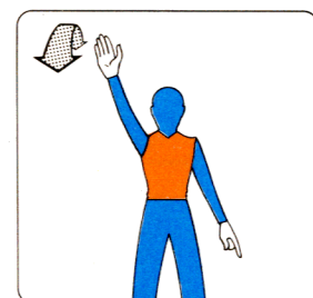
URNS WHILE BACKING - TAIL TO RIGHT POINT LEFT ARM DOWN AND RIGHT ARM BROUGHT FROM OVERHEAD, VERTICAL POSITION TO HORIZONTAL FORWARD POSITION, REPEATING RIGHT ARM MOVEMENT.
