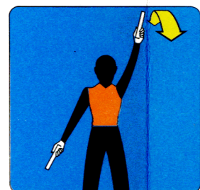
URNS WHILE BACKING-TAIL TO LEFT POINT RIGHT ARM DOWN AND LEFT ARM BROUGHT FROM OVERHEAD, VERTICAL POSITION TO HORIZONTAL FORWARD POSITION, REPEATING LEFT ARM MOVEMENT
