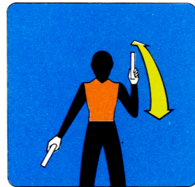
TURN TO LEFT POINT RIGHT ARM DOWNWARD, LEFT ARM IS REPEATEDLY MOVED UPWARD-BACKWARD. SPEED OF ARM MOVEMENT INDICATING RATE OF TURN.
