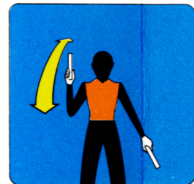
TURN TO RIGHT POINT LEFT ARM DOWNWARD, RIGHT HAND REPEATEDLY MOVED UPWARD-BACKWARD. SPEED OF ARM MOVEMENT INDICATING RATE OF TURN.
