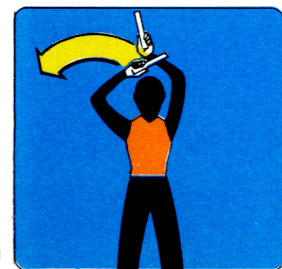
DOWN LOCKS/UNDERCARRIAGE PINS-REMOVE WITH ARMS AND HANDS IN 'INSTALL-DOWNLOCKS' POSITION, THE RIGHT HAND UNCLASPS THE LEFT FOREARM.
