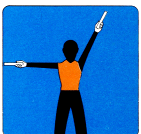
PERSONNEL - APPROACH THE AIRCRAFT LEFT HAND RAISED VERTICALLY OVERHEAD, PALM TOWARDS AIRCRAFT. THE OTHER HAND INDICATES TO PERSONNEL CONCERNED AND GESTURES TOWARDS AIRCRAFT.
