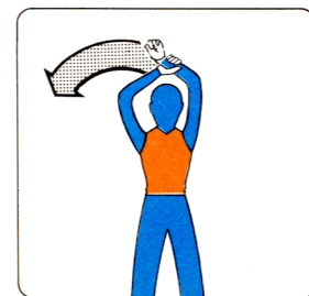
DOWN LOCKS/UNDERCARRIAGE PINS-REMOVE WITH ARMS AND HANDS IN 'INSTALL-DOWNLOCKS' POSITION, THE RIGHT HAND UNCLASPS THE LEFT FOREARM.
