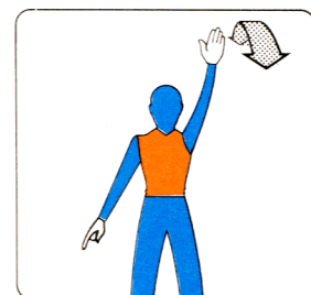
URNS WHILE BACKING-TAIL TO LEFT POINT RIGHT ARM DOWN AND LEFT ARM BROUGHT FROM OVERHEAD, VERTICAL POSITION TO HORIZONTAL FORWARD POSITION, REPEATING LEFT ARM MOVEMENT
