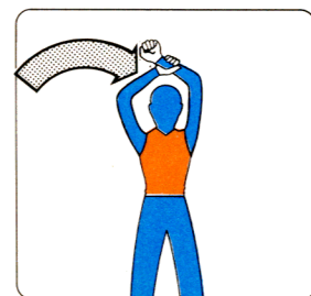
DOWN LOCKS/UNDERCARRIAGE PINS-INSTALL WITH ARMS ABOVE HEAD. THE RIGHT HAND CLASPS LEFT FOREARM AND THE LEFT FIST IS CLOSED
