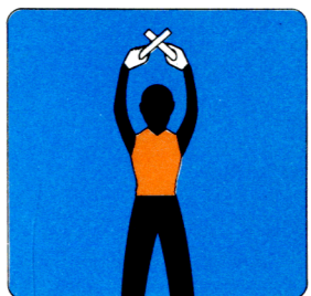
BRAKES - ON DAY - ARMS ABOVE HEAD, OPEN PALMS AND FINGERS RAISED THEN FIST CLOSED WITH PALMS TOWARD AIRCRAFT NIGHT - ARMS ABOVE HEAD, THEN WANDS CROSSED BRAKES - OFF DAY - REVERSE OF ABOVE NIGHT - CROSSED WANDS, THEN UNCROSSED
