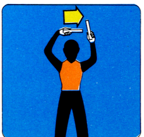
GROUND ELECTRICAL POWER SUPPLY-CONNECT HANDS ABOVE HEAD, LEFT FIST PARTIALLY CLOSED, RIGHT HAND MOVED IN DIRECTION OF LEFT HAND WITH FIRST TWO FINGERS EXTENDED AND INSERTED INTO CIRCLE MADE BY FINGERS OF THE LEFT HAND.
