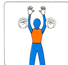
BRAKES - ON DAY - ARMS ABOVE HEAD, OPEN PALMS AND FINGERS RAISED THEN FIST CLOSED WITH PALMS TOWARD AIRCRAFT NIGHT - ARMS ABOVE HEAD, THEN WANDS CROSSED BRAKES - OFF DAY - REVERSE OF ABOVE NIGHT - CROSSED WANDS, THEN UNCROSSED
