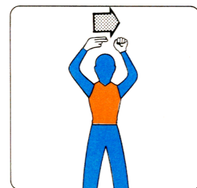
GROUND ELECTRICAL POWER SUPPLY-CONNECT HANDS ABOVE HEAD, LEFT FIST PARTIALLY CLOSED, RIGHT HAND MOVED IN DIRECTION OF LEFT HAND WITH FIRST TWO FINGERS EXTENDED AND INSERTED INTO CIRCLE MADE BY FINGERS OF THE LEFT HAND.
