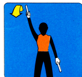
URNS WHILE BACKING - TAIL TO RIGHT POINT LEFT ARM DOWN AND RIGHT ARM BROUGHT FROM OVERHEAD, VERTICAL POSITION TO HORIZONTAL FORWARD POSITION, REPEATING RIGHT ARM MOVEMENT.
