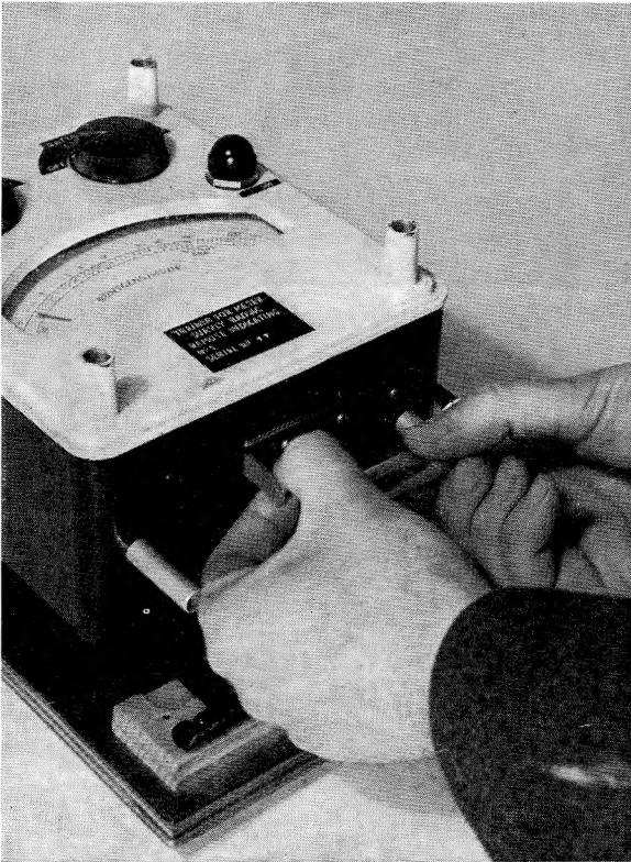
Fig. 5. Feeding pattern into the intake slot
