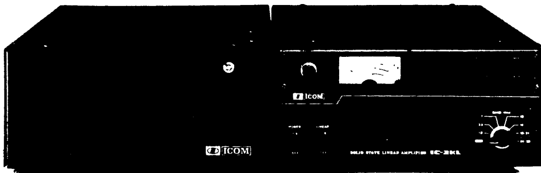
Fig 3 MCPA Linear Amplifier
