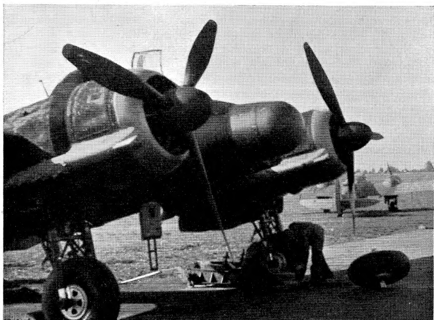
Perspex Nose Housing the Scanner
