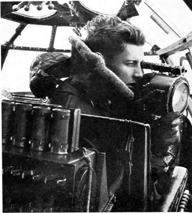
A recognition signal is flashed by Aldis lamp as soon as aircraft makes contact with convoy.
