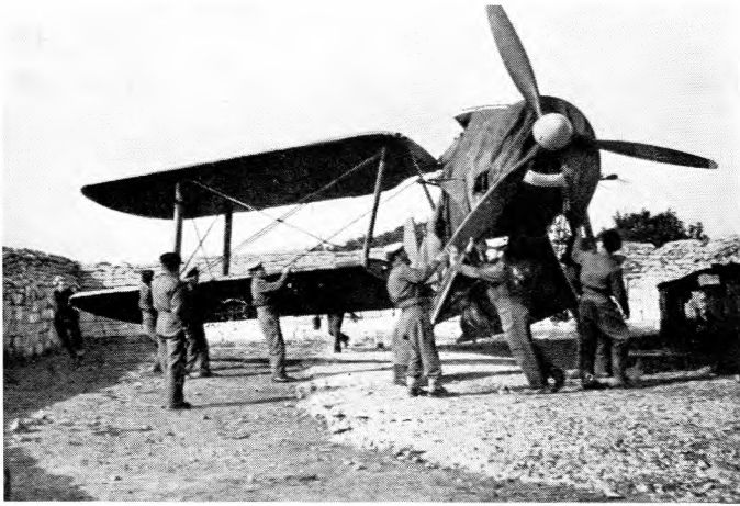
OFF TO STRIKE FROM MALTA. Naval ratings unfold the wings of an Albacore standing in its pen at an R.A.F. Station in Malta. The pen gives protection against the blast from enemy bombs.
