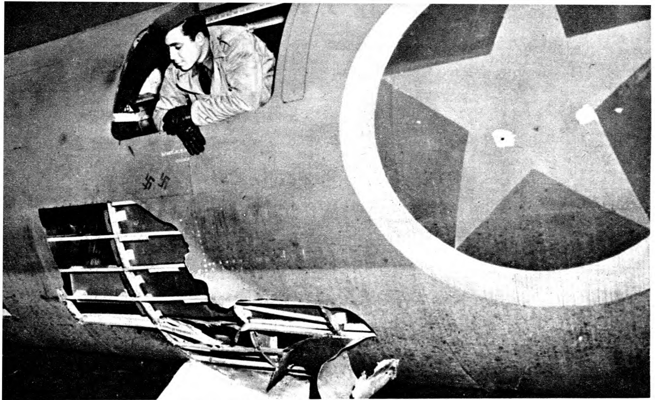
Battle damage: a German 20-mm. shell peeled the metal covering off this bomber like skin off an onion.
