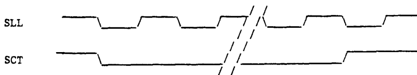
FIGURE 3.17: TYPICAL LINE AND FRAME OUTPUT SIGNALS
