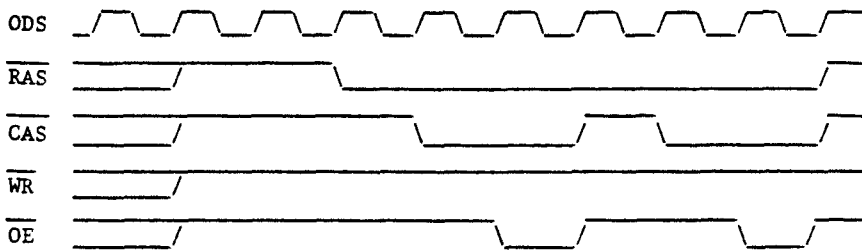
FIGURE 3.14: DOUBLE READ ACCESS (DISPLAY)
