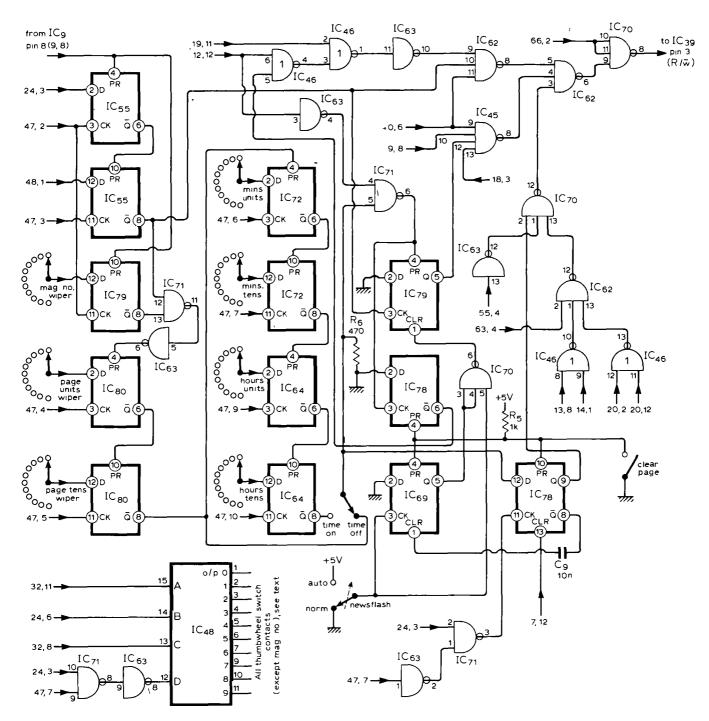
It will be noticed from the circuit diagram that the clear input of  $IC_{79}$  is fed from the output of (70, 6). However, this only has any effect in the autonewsflash mode of operation which will be dealt with later. During normal operation the clear input is held at 1 because one input of (70, 6) is held at 0 by the auto/normal switch.
