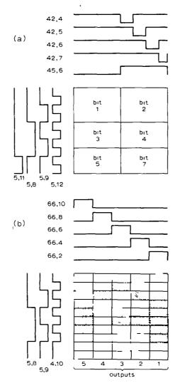
Fig. 2 (a) Graphic character segments are of unequal sizes to avoid gaps between characters. Alphanumeric generation is shown at (b), which does not include the three vertical columns for gaps between characters.
