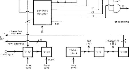
Fig. 8. A typical output processor.
