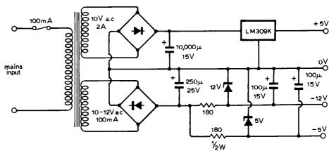
Fig. 4. A suggested power supply circuit.
