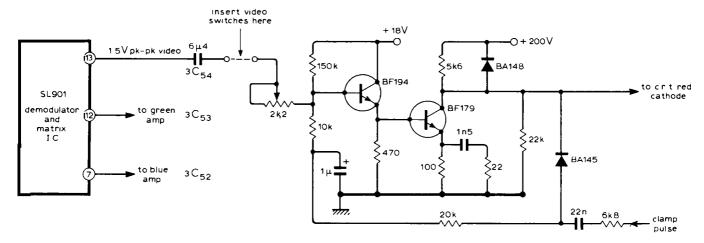
Fig. 2 Video output circuitry of the Bush CTV182S, CTV184S and CTV187CS
