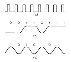
Fig. 2. The non-return-to-zero method of transmitting binary information is at (b) with the attendant clock at (a). A succession of 101010 etc. gives a half-clock frequency waveform and, if the pulse shape is a raised cosine, as used in Teletext, the result is a sinusoid at 3.5 MHz.
