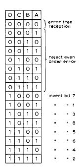
A,B,C & D are parity checks over the following bit no's
