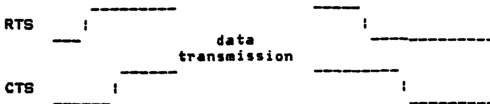
Figure 3-1 RS232C Transmission Cycle
