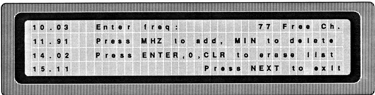
Figure 3-6b. Narrowband Frequency List, Entry Procedure
